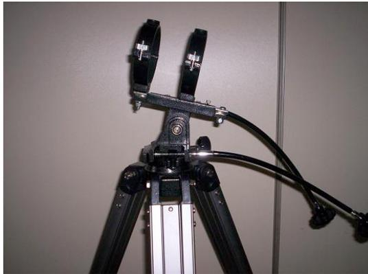
The **Altazimuth Mount** (sometimes called alt-az) is the simplest type of mount with two motions, altitude (vertical) and azimuth (horizontal): thus the name Altazimuth.
